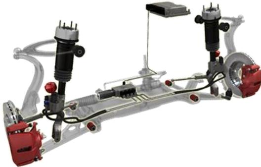
Fig. 5 Active suspension layout.
